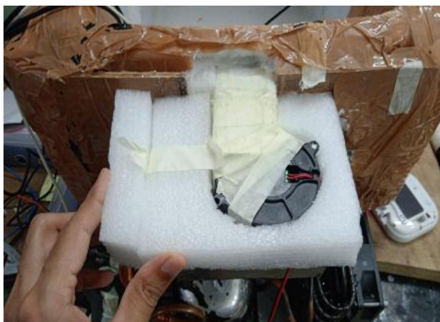
Figure 10: Radial blower type Evaporator Assembly
