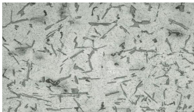
Figure 6: The microstructure of a composite cast with 12 wt.% reinforcement using a copper chill.
