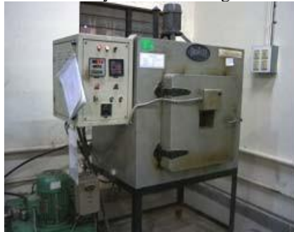
Fig 3: Post curing oven Casting Produced
