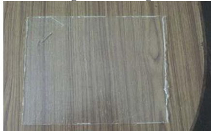
Fig 4: Neat Resin casting Preparation of Casting with Multi Walled Carbon Nano Tubes
