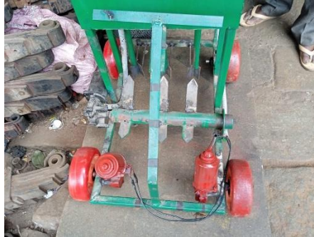
Figure 6: Rotor shaft and weeder blades
