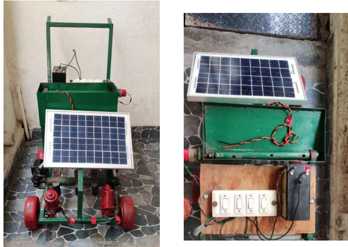
Figure 1: Prototype build of solar weeder
