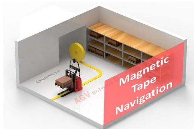
**Fig.3-Magnetic Tape Navigation.[3]**
