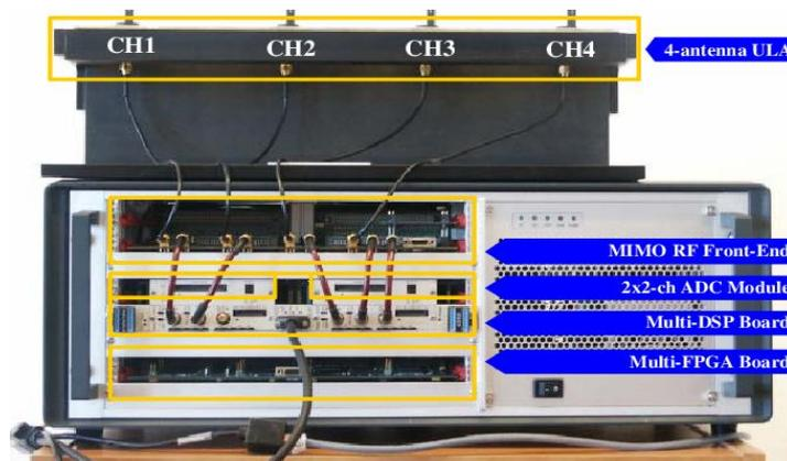
Fig. 8- Multi-Antenna Dual-band Receiver setup.[7]
