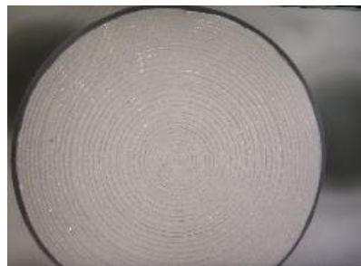
Figure 1 microstructure of Ti6Al4V before micro blasting
