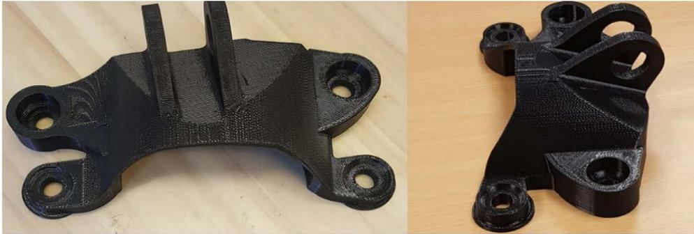
Figure 6. Engine Bracket after Fused Deposition Modelling (Additive Manufacturing) [16]
