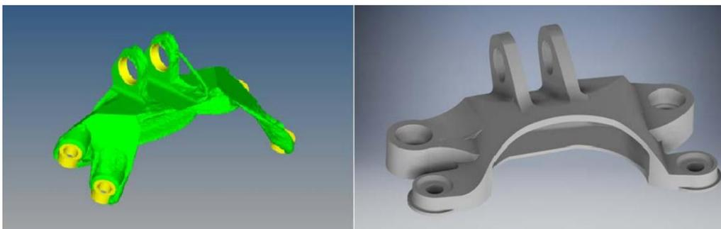
Figure 5. Optimal Geometry and Remodeled design [25]
