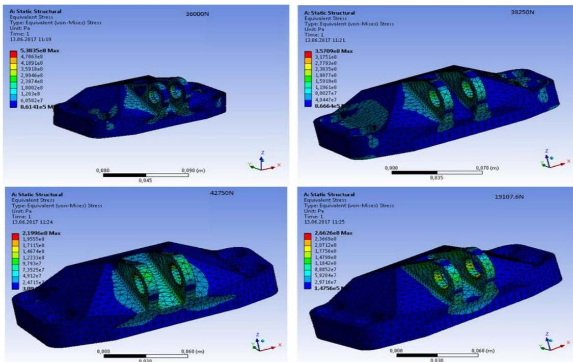
Figure 4. Von Mises distribution contour plot marked by blue [16]
