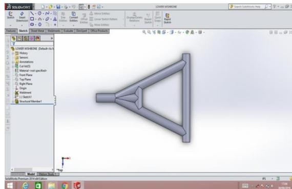
Design of upper and lower wishbones in Solid Works
