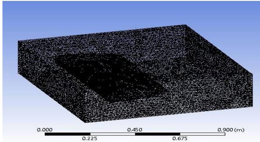
**Figure 4:** Unstructured Mesh of Spoiler - Tetrahedron Cell shape (All dimensions are in m)
