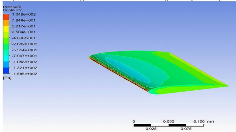
**Figure 8:** Pressure distribution over the full span of airfoil shaped spoiler (All dimensions are in m)
