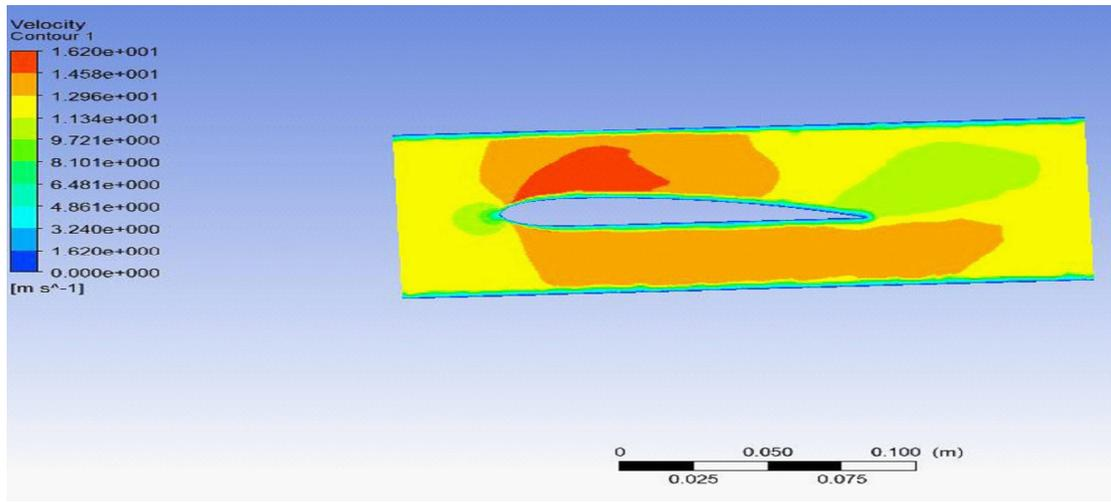
**Figure 7:** Velocity distribution over the cross section of spoiler (All dimensions are in m)
