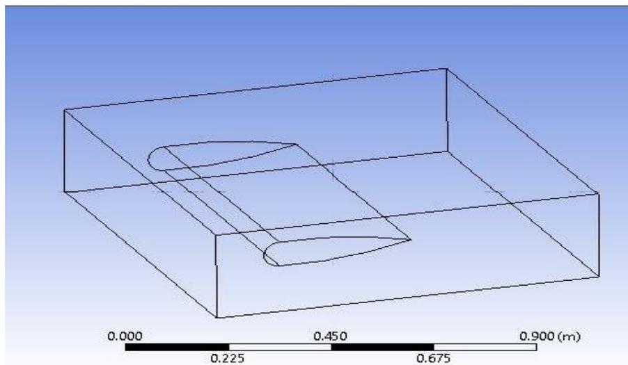
**Figure 3:** Spoiler geometry is imported into ansys and boundary enclosure is done (All dimensions are in m)
