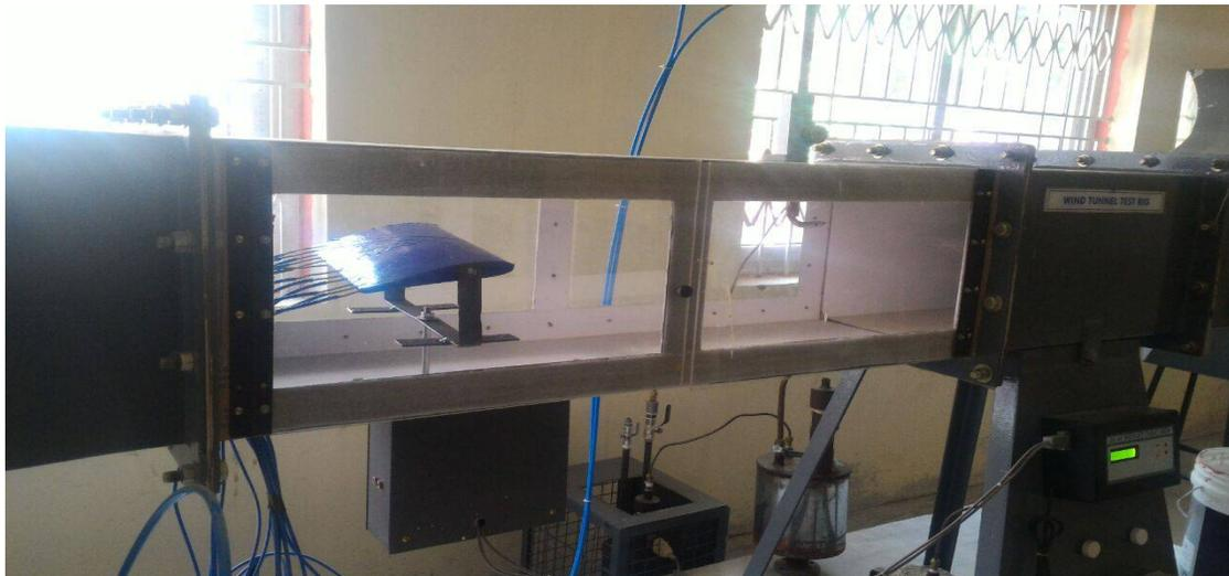
**Figure 9:** Wind Tunnel testing of Airfoil shaped spoiler scaled model
