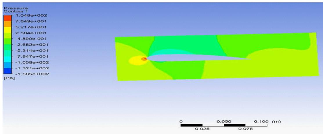
**Figure 6:** Pressure distribution over the cross section of spoiler (All dimensions are in m)
