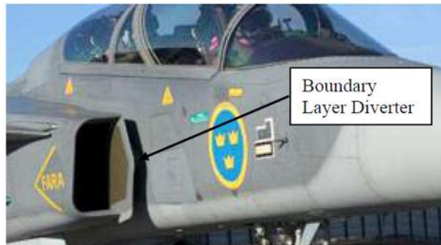
Figure 1 : JAS 39 Gripen with boundary layer bleed
