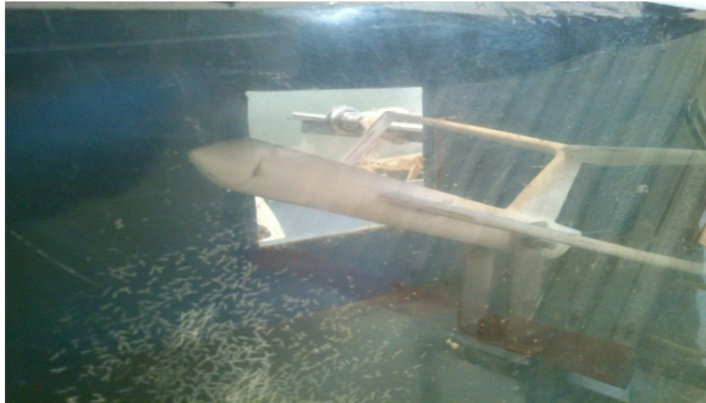
Figure 4. Mounting of model in wind tunnel.
