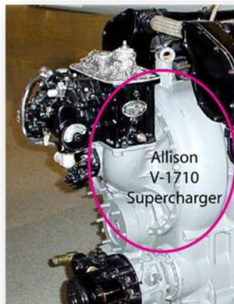
Figure 4: Allison V-1710 with Single-Stage Supercharger
