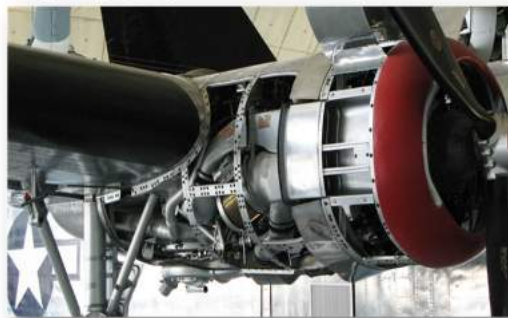
Figure 5: Turbocharger tubing in a bomber engine
