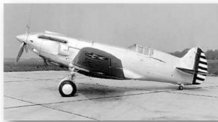
Figure 7: XP-37 with second-stage turbocharger
