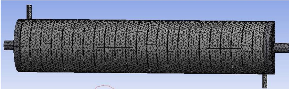
Figure 5.1 the mesh generated for the Geometry of the shell and tube Heat Exchanger
