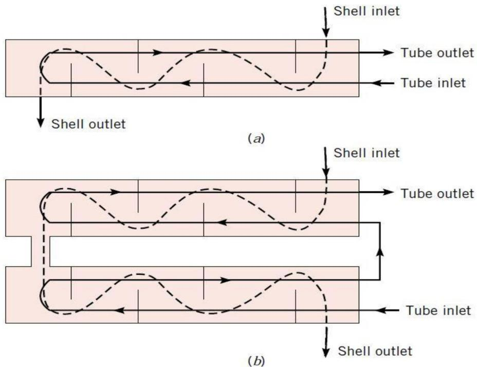
Figure-2 Shell-and-tube heat exchangers. (a) One shell pass and two tube passes. (b) Two shell passes and four tube passes.
