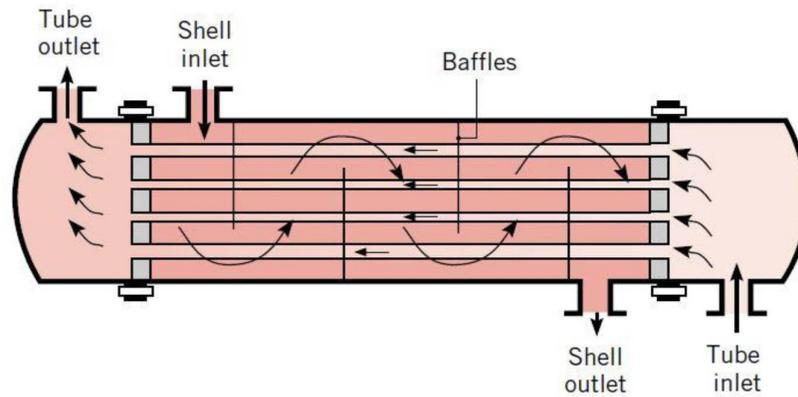
Figure-1. Shell-and-tube heat exchanger with one shell pass and one tube pass (cross-counter flow mode of operation)
