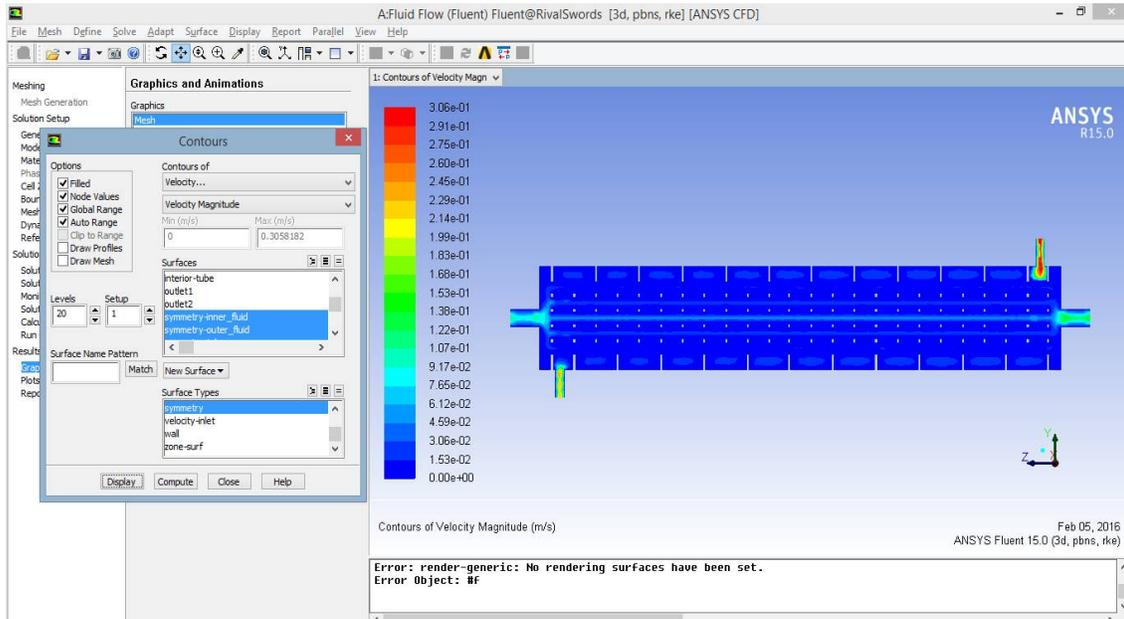
Figure 5.5: Velocity Contour Plot at Symmetrical Plane
