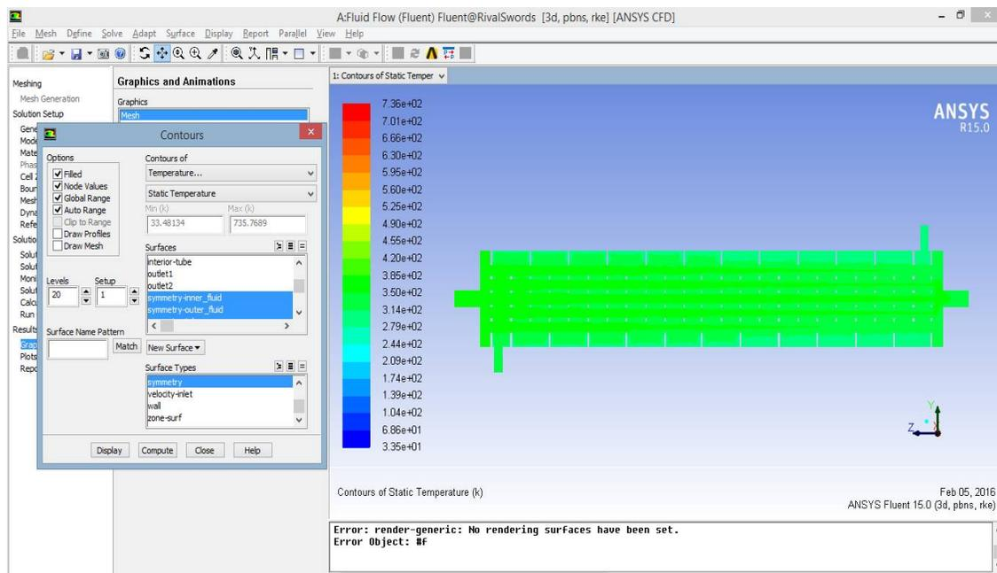
Figure 5.4: Temperature Contour Plot at Symmetrical Plane
