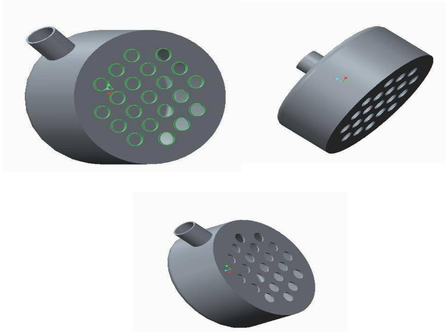
Figure4. Different header configurations of the shell-and-tube type heat exchanger.
