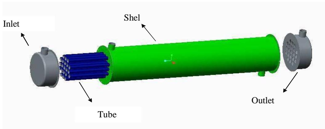
Figure 4.1 Shell and tube heat exchanger original geometry
