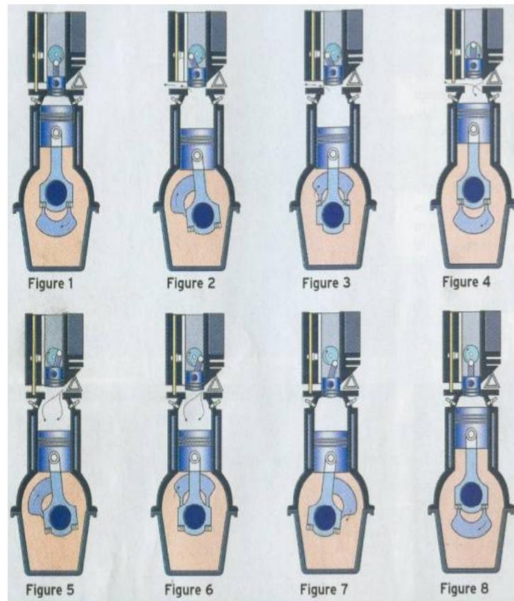
*Fig2: Six stroke engine & their working function*
