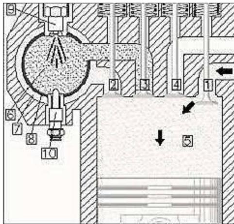
Fig 1: Components of Six Stroke Engine
