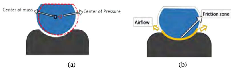
Figure 2. (a). Unbalance between center of mass and center pressure. (b) airflow friction (Figueiredo 2013)
