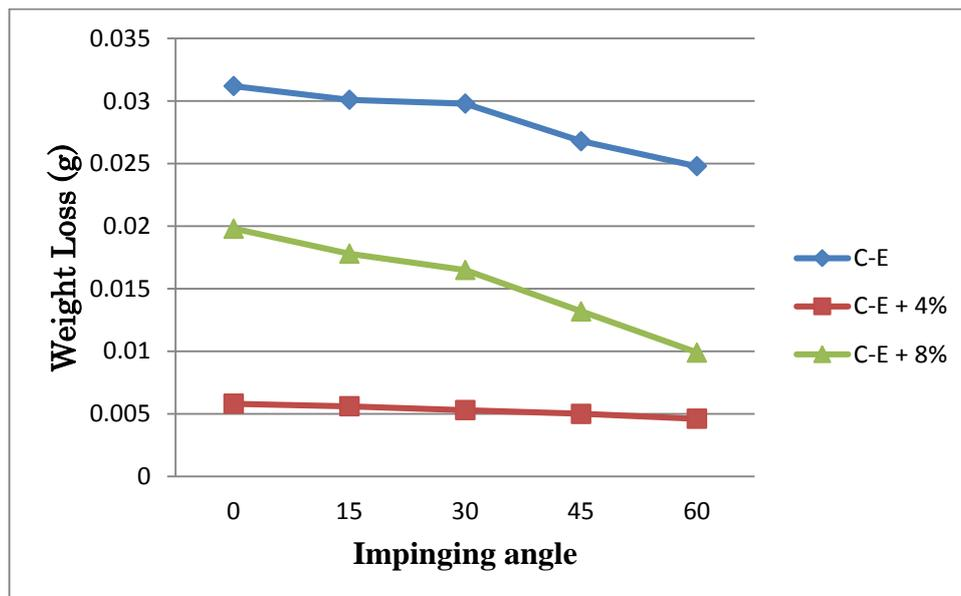
**Fig 4.1:** Weight loss Vs Impinging angle for C-E composites – Without ageing
