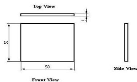
**Fig 3.1.** Air Jet Erosion Test Specimen
