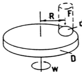
Figure shows Schematic Diagram of Pin on Disc Test Where,
