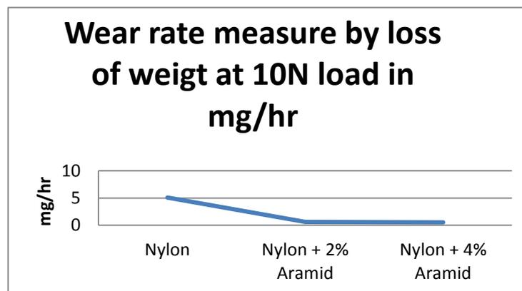
**Graph1:** Pin on Disc test result at 10N load.
