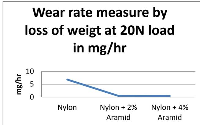
**Graph2:** Pin on Disc test result at 20N load.
