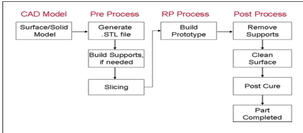
**Fig 1.** Flow Chart for RP Components
