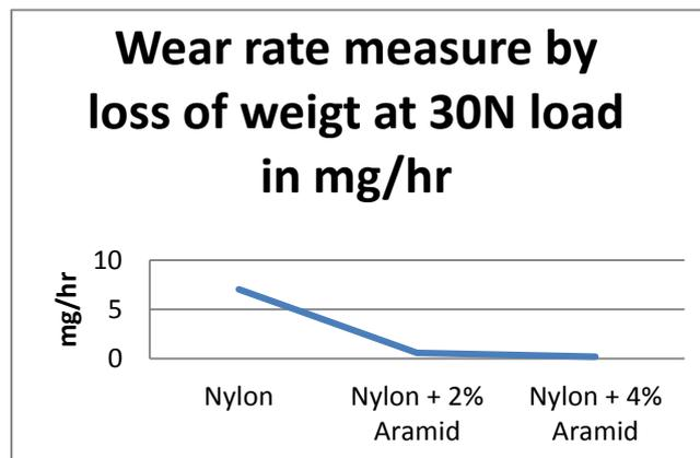
**Graph3:** Pin on Disc test result at 30N load.
