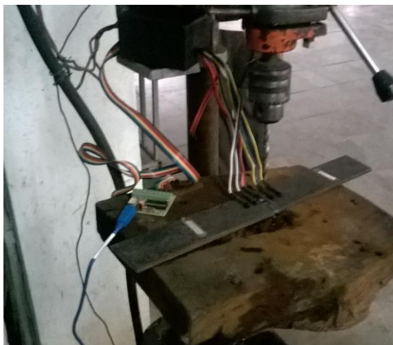
Fig.5(a). The strain gauges are bonded to the specimen
