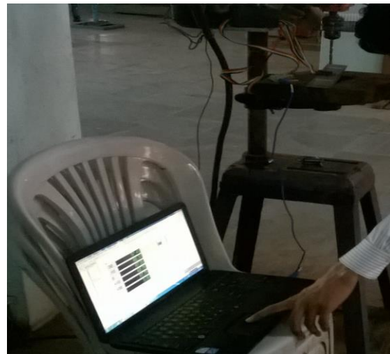
Fig.5 (b). Strains are measured by Multi Channel Strain Indicator
