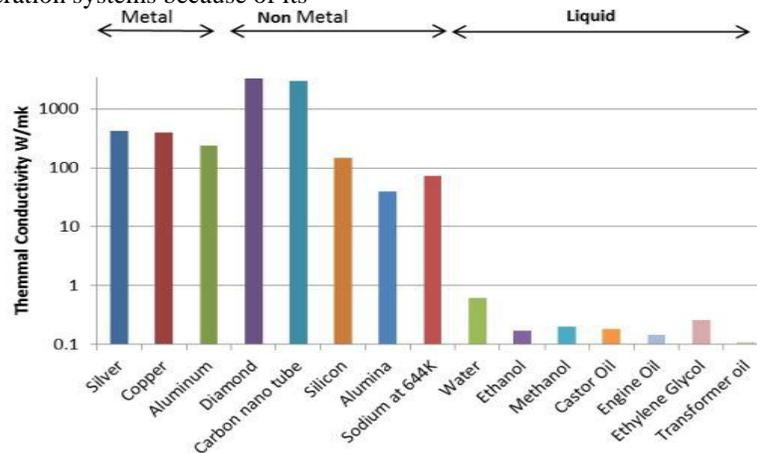
Fig: 1 - Comparison of Thermal Conductivities of Different Materials
