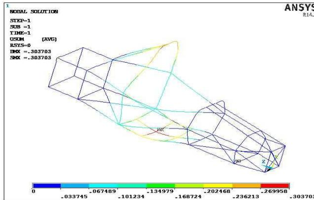
Fig 14: Deformation during Acceleration test (load applied in the driver cabin and apply to the structure in backward direction)
