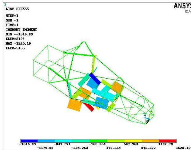
Fig 11: Bending moment during vertical bending test (load applied at driver cabin)
