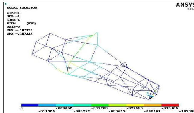
Fig 12: Deformation during lateral bending test
