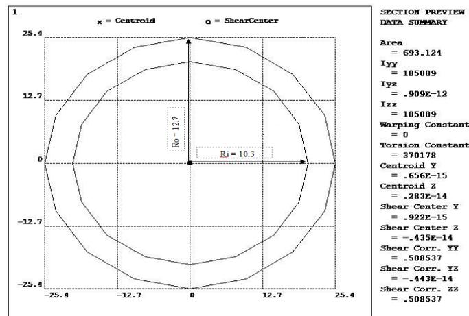
Fig 6: Main and front roll hoop cross sectional area of a chassis frame
