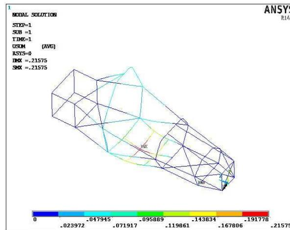
Fig 10: Deformation during vertical bending test (load applied at driver cabin)
