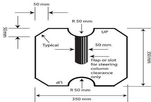
Fig 4: Foot-well clearance template
