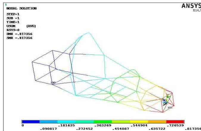
Fig 8: Deformation during longitudinal torsion (load applied at bulk head)
