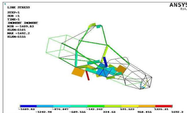
Fig 15: Bending moment during Acceleration test (load applied in the driver cabin and apply to the structure in backward direction)
