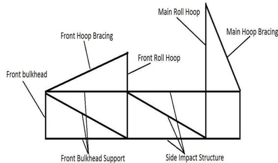
Fig 1. Pictorial representation of the members required by the FSAE rules.
