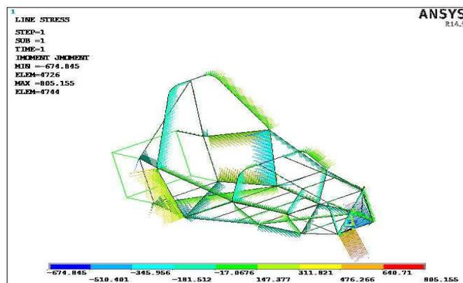
Fig 9: Bending moment during the longitudinal torsion (load applied at bulk head)
