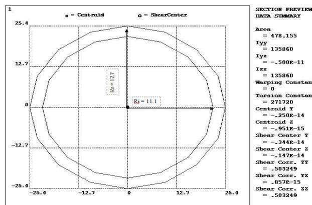
Fig 7: Other sectional members cross sectional area of a chassis frame
