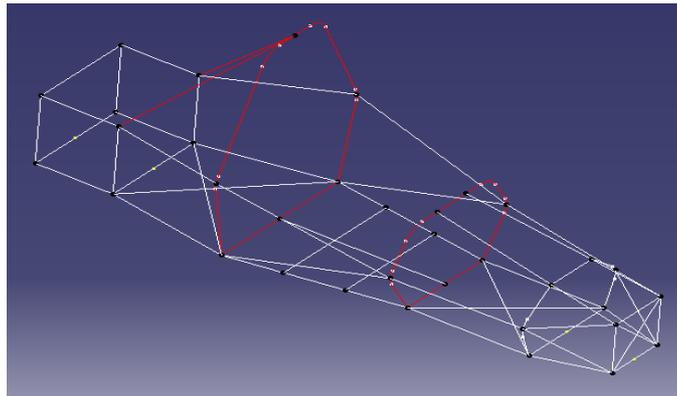
Fig 5: 3D Chassis frame
