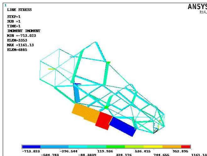
Fig 13: Bending moment during lateral bending test
