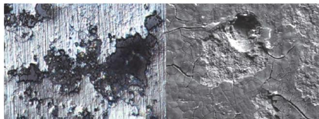
Fig. 4. SEM images showing the pitting corrosion for propeller
