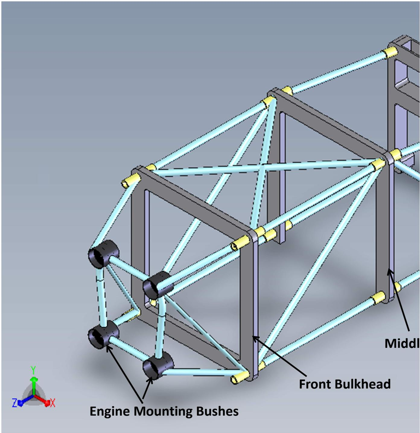
Fig 1 Model of the Interfacing frame
