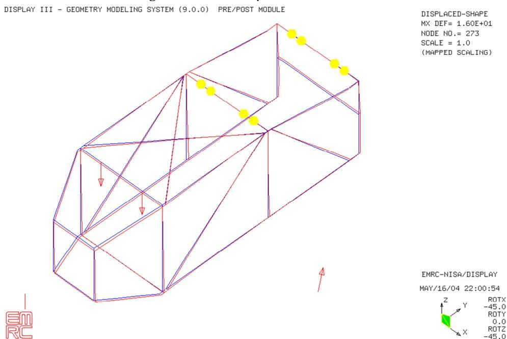
Fig 5 Displacement plot for Load Case – 2
