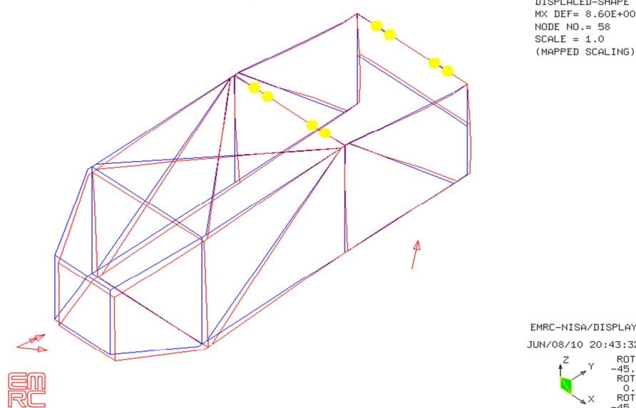
Fig 3 Displacement Plot for Load Case - 1
