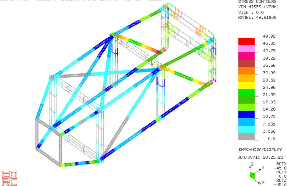
Fig 2 Stress Contour Plot for Load Case - 1
