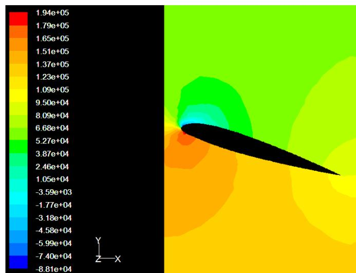
**Fig 9.** Contours of static pressure at 17 degree AoA
