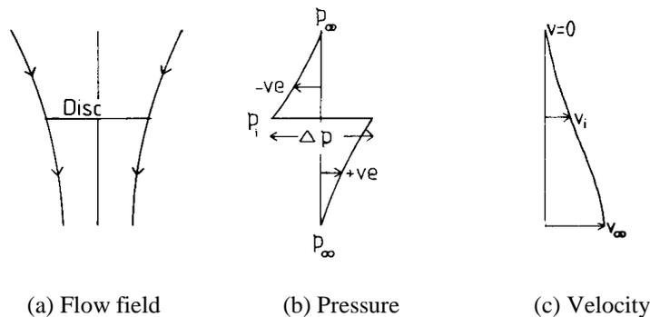
In equation (1), ' $\rho$ ' is the air density, and using the Actuator disc concept for rotor in hover the outflow becomes
