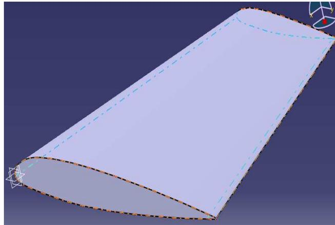
**Fig 5.** CATIA Model prepared using NACA –23012 airfoil
