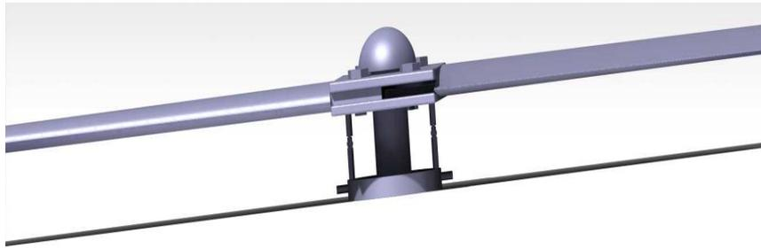
**Fig 6.** Assembled rotor blades with hub, bracket and pins
