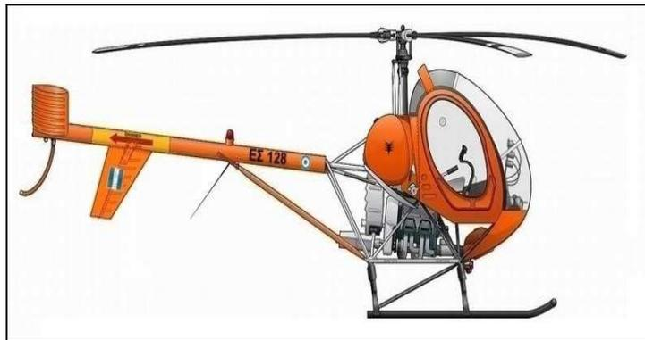
**Fig 1.** Rotor craft with single main rotor design
