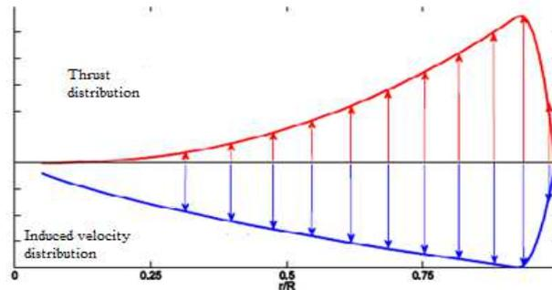
**Fig 4.** Distribution over a symmetrical blade with constant pitch angle
