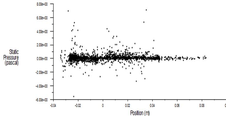
**Fig 10.** Static Pressure Variations from Root to Tip of the blade
