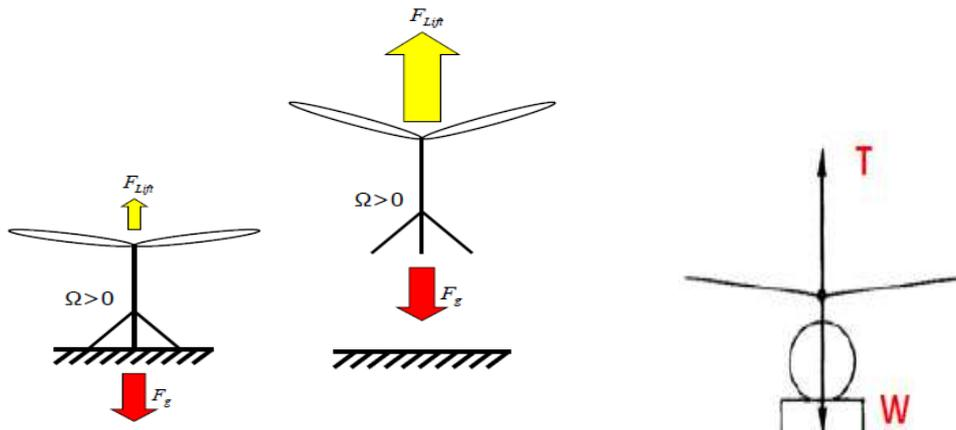
**Fig 2. Forces on the rotor head and hovering layout**
