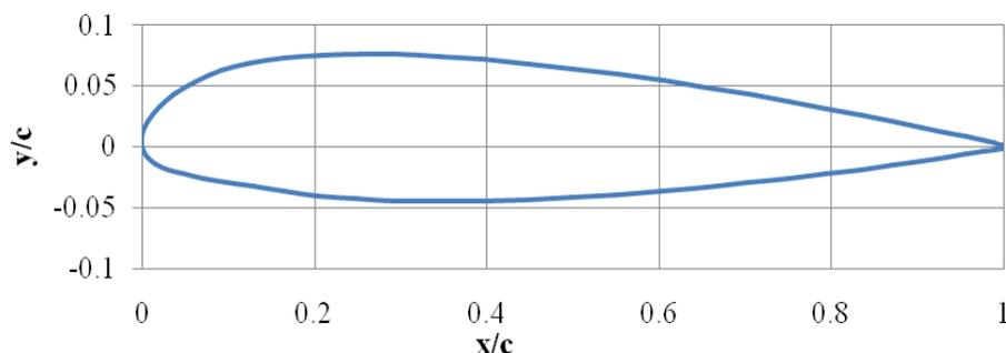
**Fig 3. Constructed NACA 23012 Airfoil in the solver**
