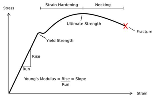
Figure 1: Typical stress vs strain diagram with the various stages of deformation
