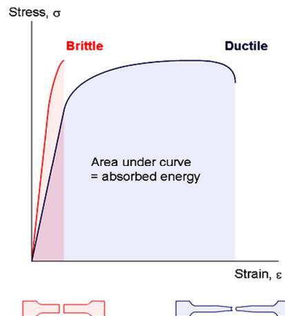
**Figure 2: Brittle vs Ductile Stress Strain Behavior**
