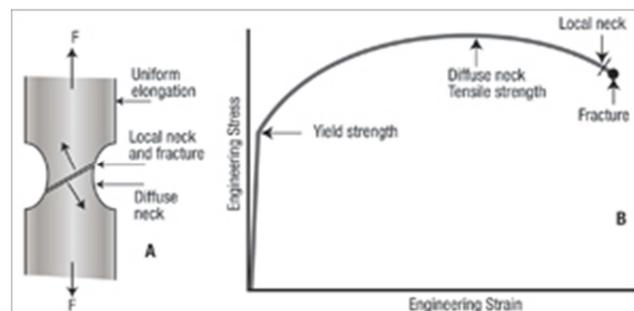
Figure 5: Schematic of a tensile-test sample (A) showing an angular local neck at the onset of fracture, and a stress-strain curve (B) with the local neck occurring just prior to the onset of specimen fracture
