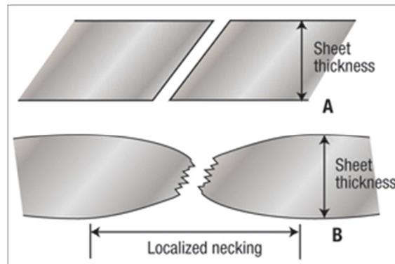
Figure4: Fracture profiles of brittle fracture (A) without any through-thickness thinning, and ductile fracture (B) showing extensive localized thinning.
