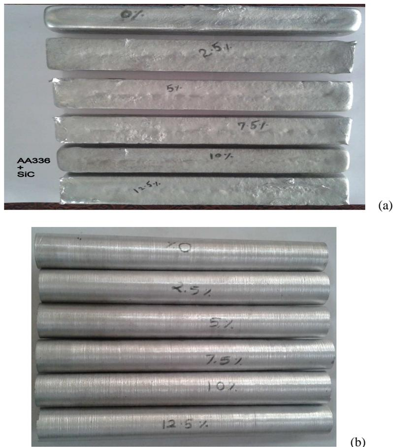
**Figure 4:** Samples with different reinforcements of SiC (blanks (a) and rods (b))
