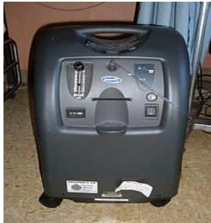
Figure2. Oxygen concentrator.
