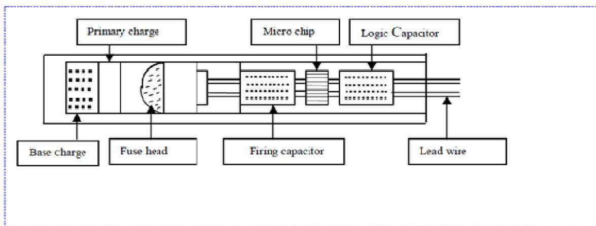
**Figure 2.6: Electronic detonator**
