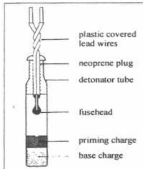
Fig 2.2 Instantaneous Electric Detonator
