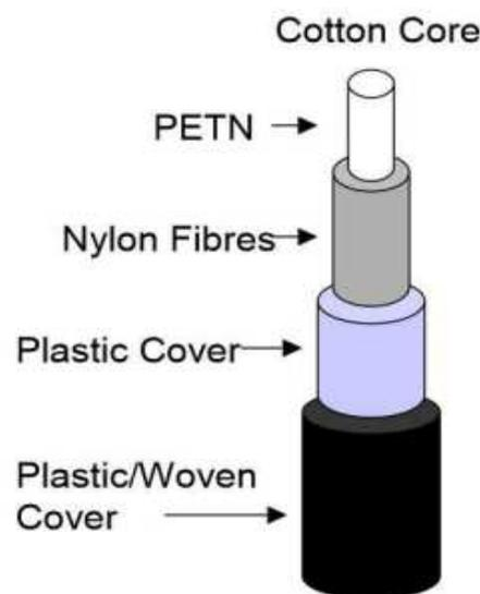
Fig2.4 Detonating Cord Make
