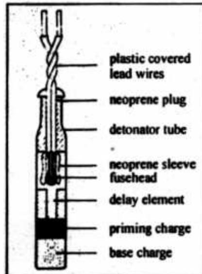
Fig 2.3 Delay Electric Detonator
