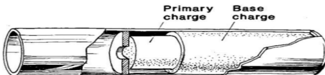
Fig 2.1 Plain detonator cross section
