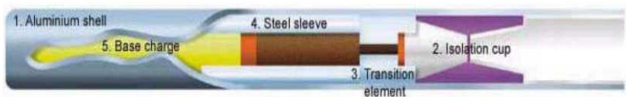
Fig2.5 NONEL Detonator Cross Section
