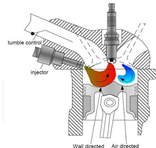
(Figure.7 Air-wall guided combustion system )
