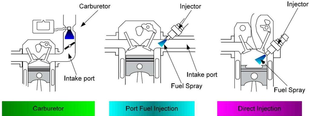
(Fig.1 Mixture formation in different fuel supply systems)
