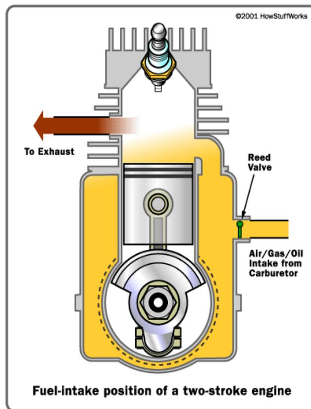
**Fig 1.1 Two stroke engine**
