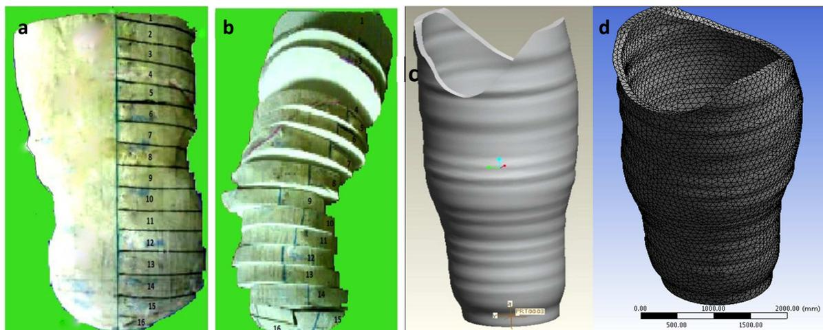
**Figure 1:** (a) Positive mold of prosthetic socket, (b) Discs of positive mold, (c) Pro-e model of prosthetic socket, (d) Mesh view of prosthetic socket
