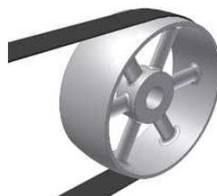
Figure-3.4 Belt and pulley
