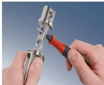
Figure-1.2 Manual deburring
