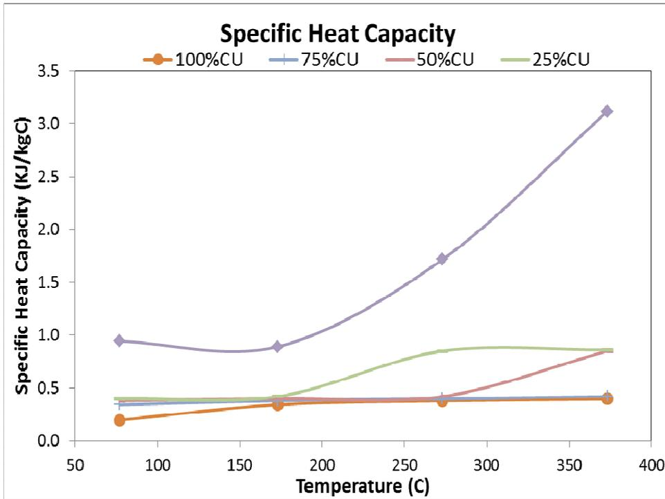
Fig.5: Sample's Specific Heat Capacity
