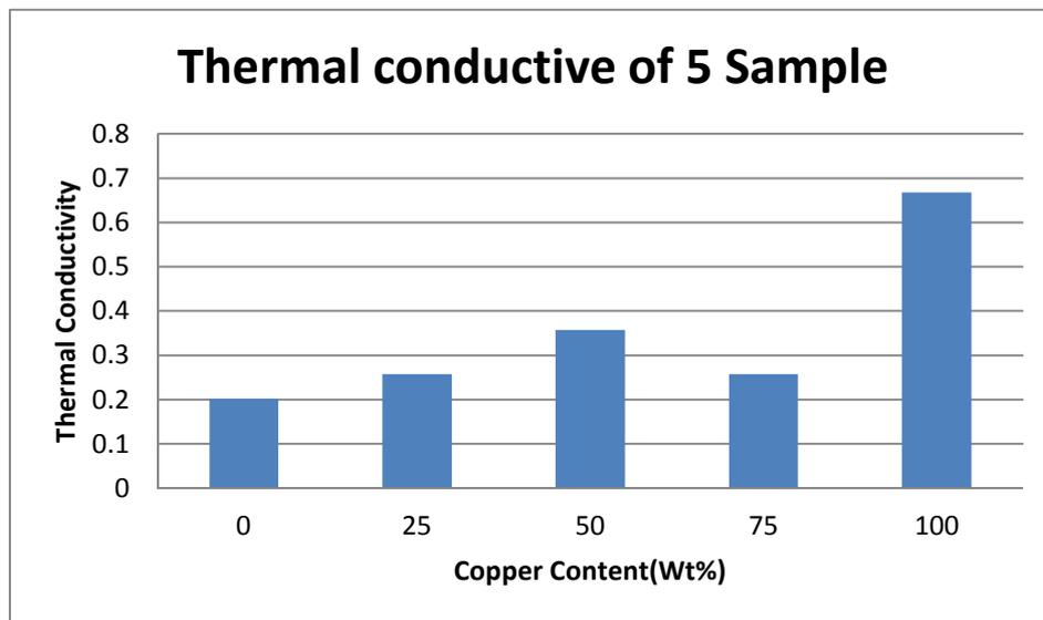
Fig.4: Thermal conductivity of specimens at 55°C.
