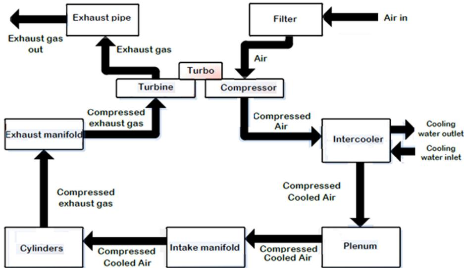
Figure 1: Flow Chart of Intake System
