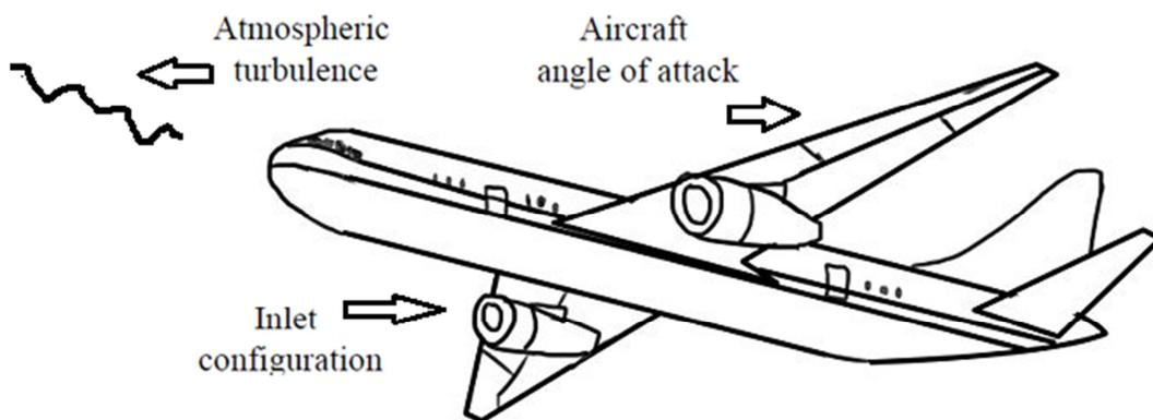
Figure 2: Inlet Total Pressure Distortions and its Configuration
