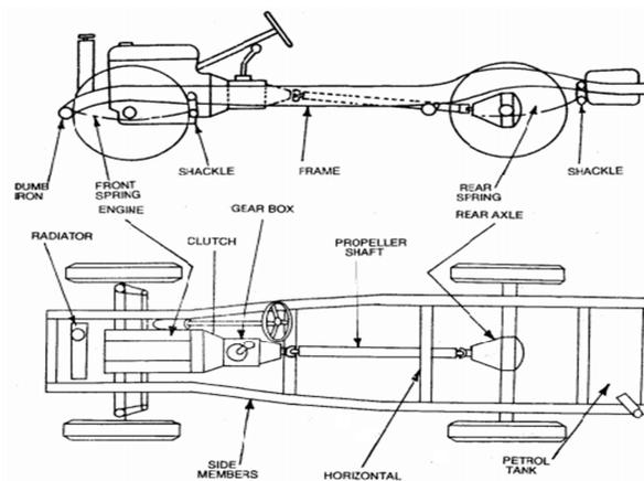
*Fig 1.1 a general Layout of Chassis and its main Components*
