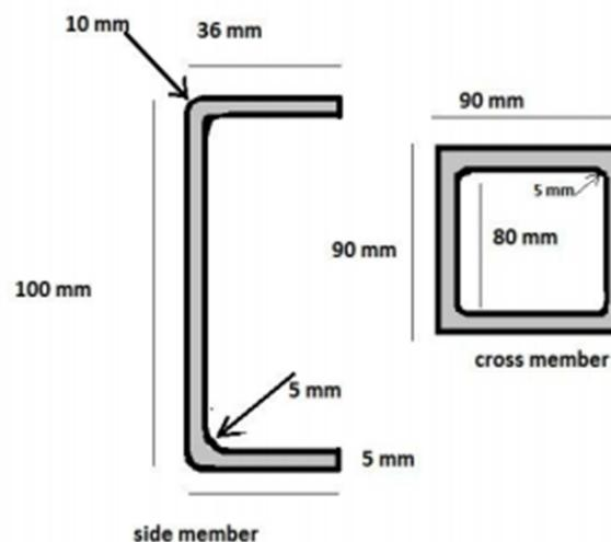
Fig 3 Dimensions of chassis using by *Manpreetsinghbajwa et.al.(2013)*
