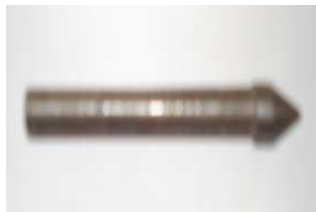
Fig.1 (a) form drilling tool
