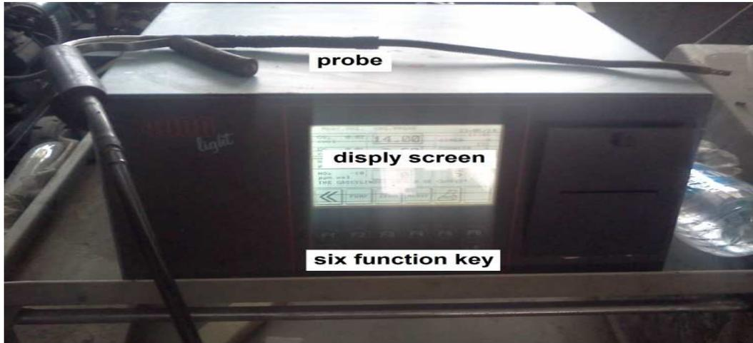
**Figure.3.** Photographic view of exhaust gas analyzer.
