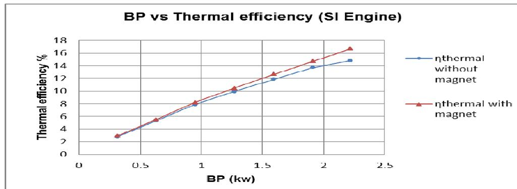
Figure.5.Variation of thermal efficiency with brake power
