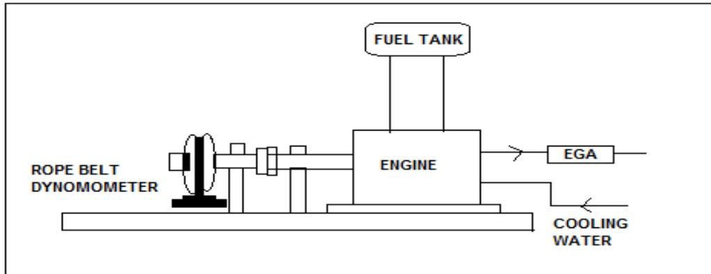
**Figure.2.** Schematic view of 1-cylinder 4-stroke SI engine
