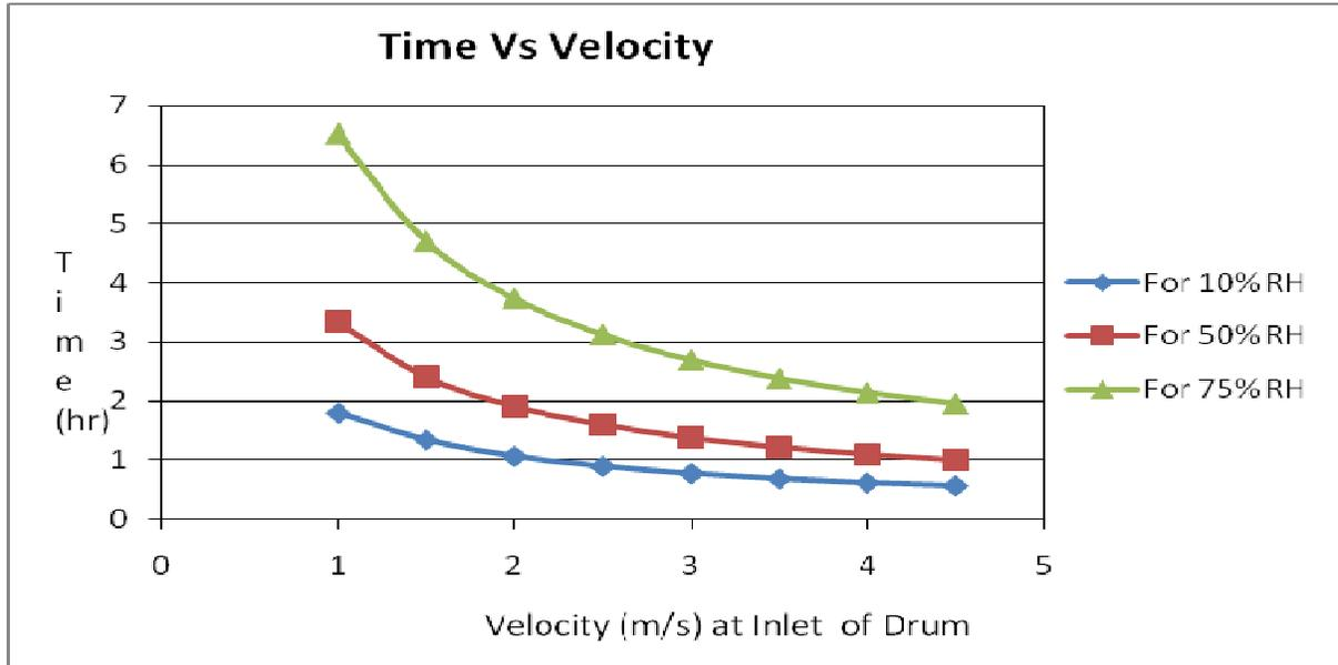
Figure 7.5 Time variation along Velocity at Inlet of drum
