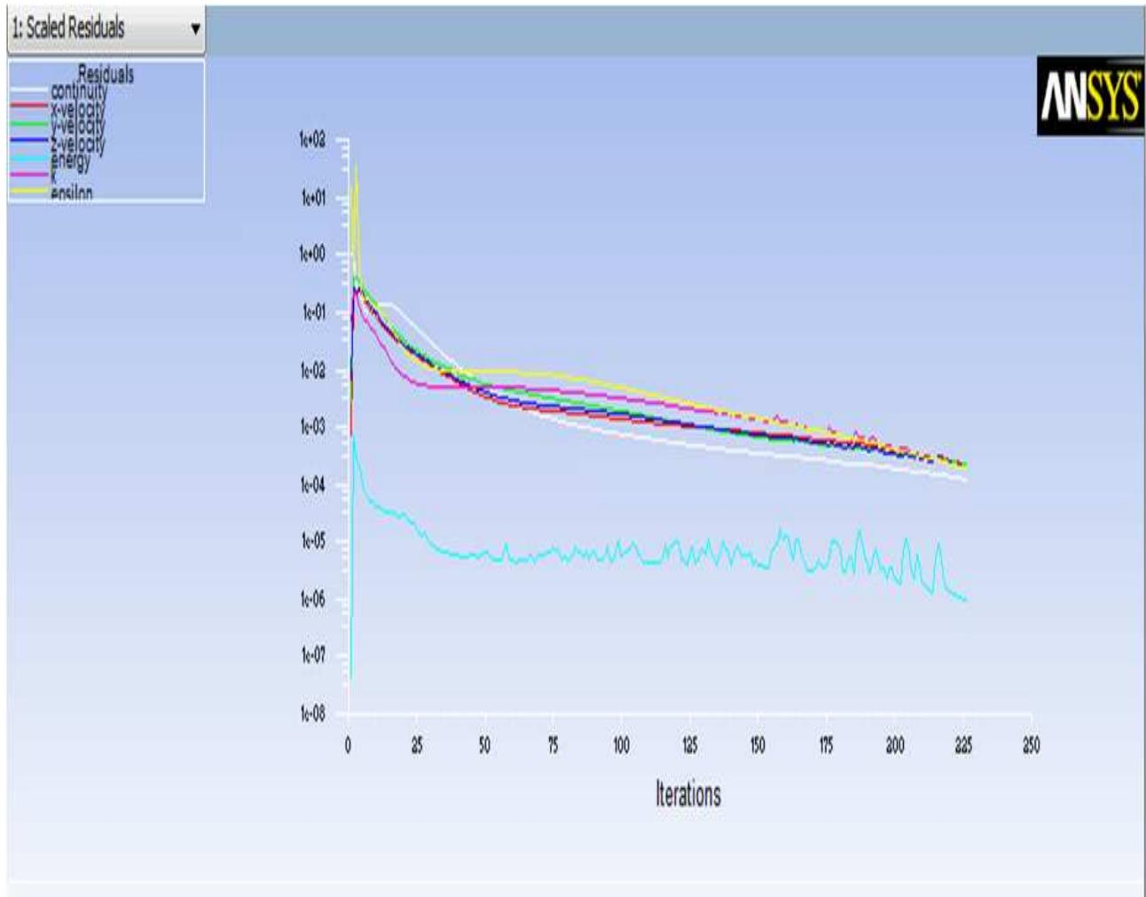
Figure 7.4 Residual plot of solution
