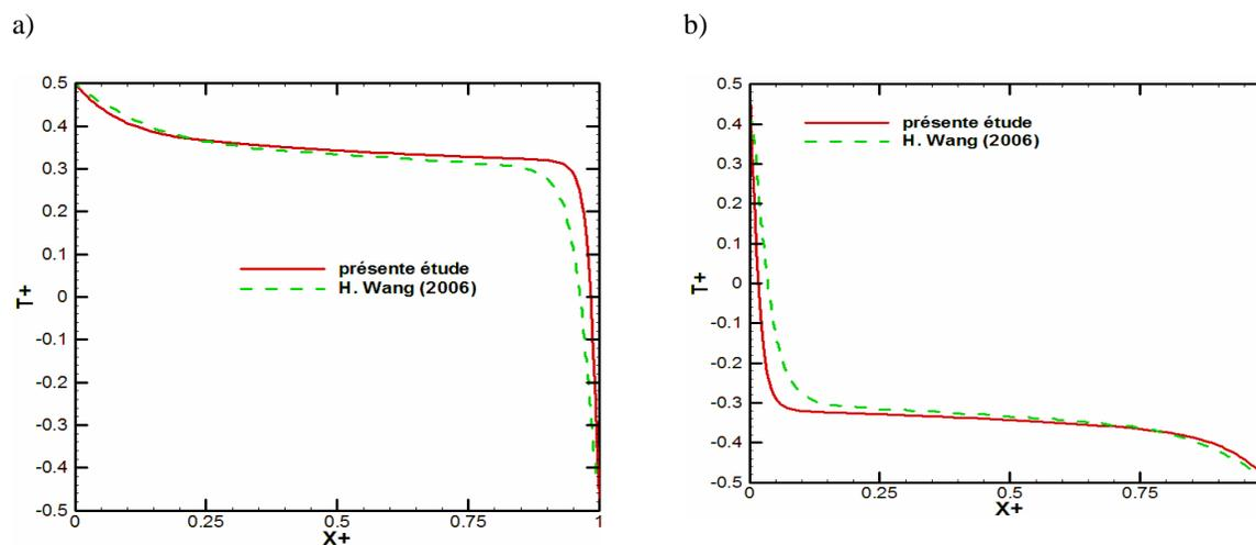
**Figure 13:** Temperature profiles for  $Ra = 10^6$ . a): on the ceiling; b): on the floor.
