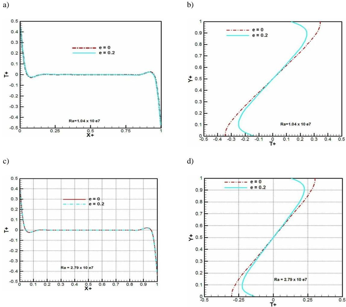
**Figure 7:** Temperature profiles at the middle of cavity for different emissivity. a) and b): at the medium height; c) and d): at the medium length.
