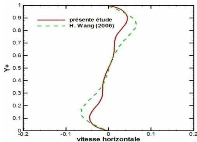
**Figure 15:** Velocity profile at the medium length of the cavity for  $Ra = 10^6$
