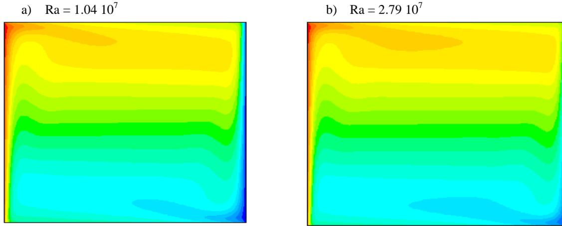
Figure 5: Thermal field with surface radiation
