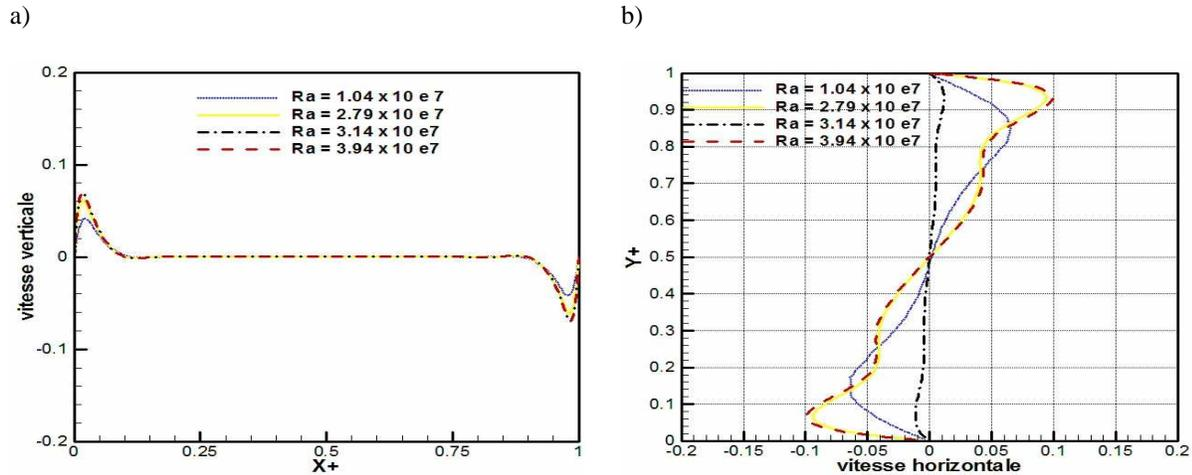
Figure 9: Vertical (a), and horizontal (b), velocities profiles at the medium length (b) and medium height (a).
