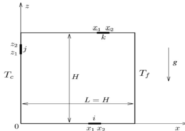
**Figure 1:** Physical domain of the square cavity:  $T_0 = (T_c + T_f)/2$  and  $T = T_c - T_f$ .
