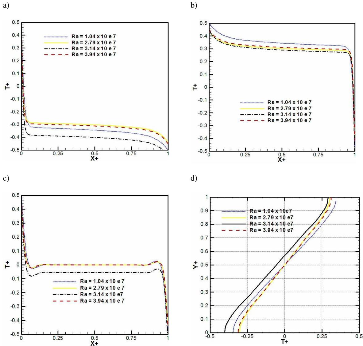
**Figure 4:** Temperature profiles for different Rayleigh numbers. a): near the lower wall, b): near the higher wall, c) and d): at the middle of the cavity
