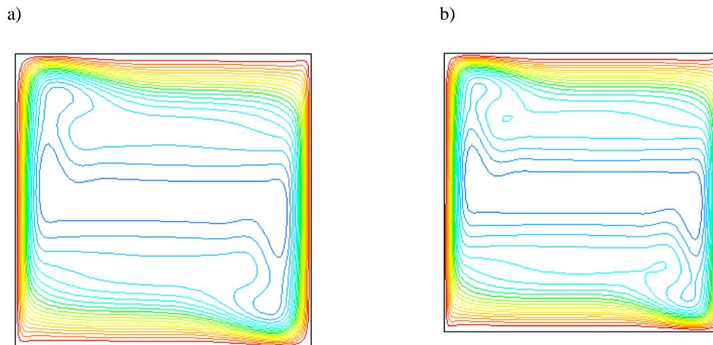
Figure 10: Dynamic field with surface radiation. a): Ra = 1.04 x 10<sup>7</sup>, b): Ra = 2.79 x 10<sup>7</sup>
