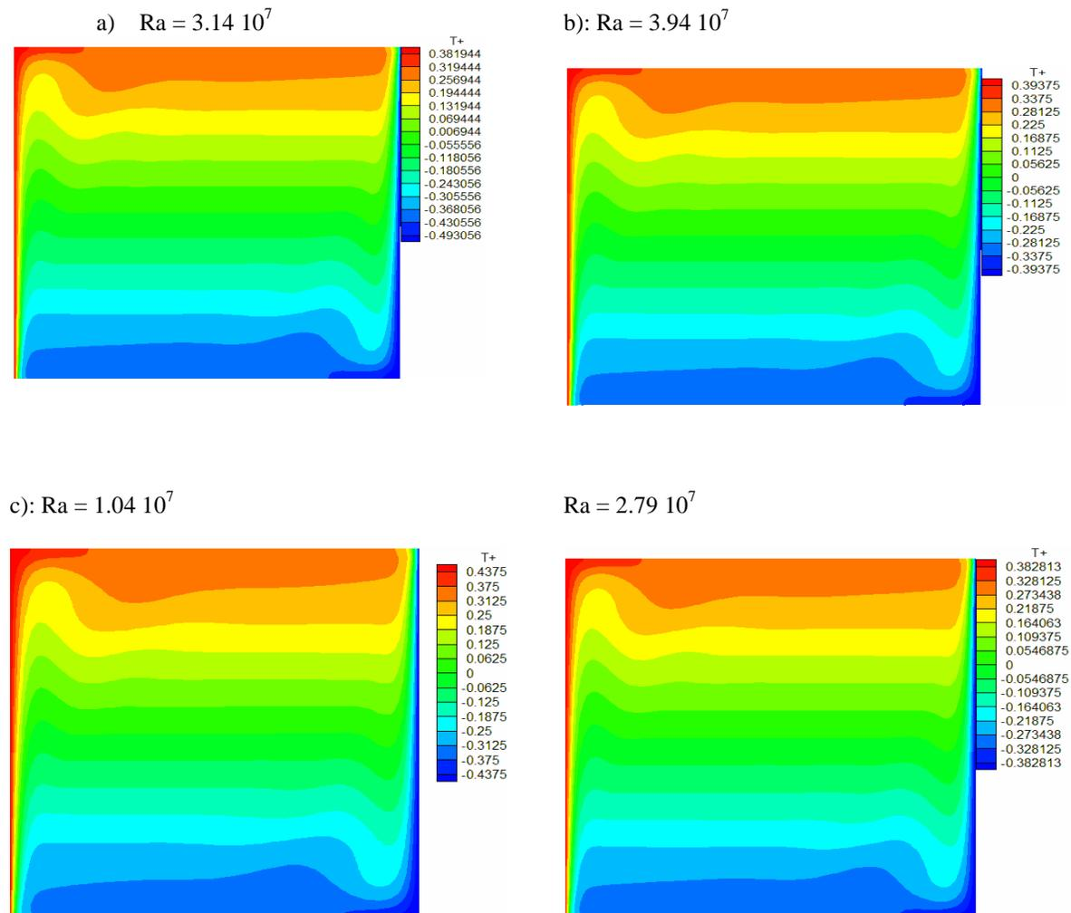
**Figure3:** Thermal field for different Rayleigh numbers
