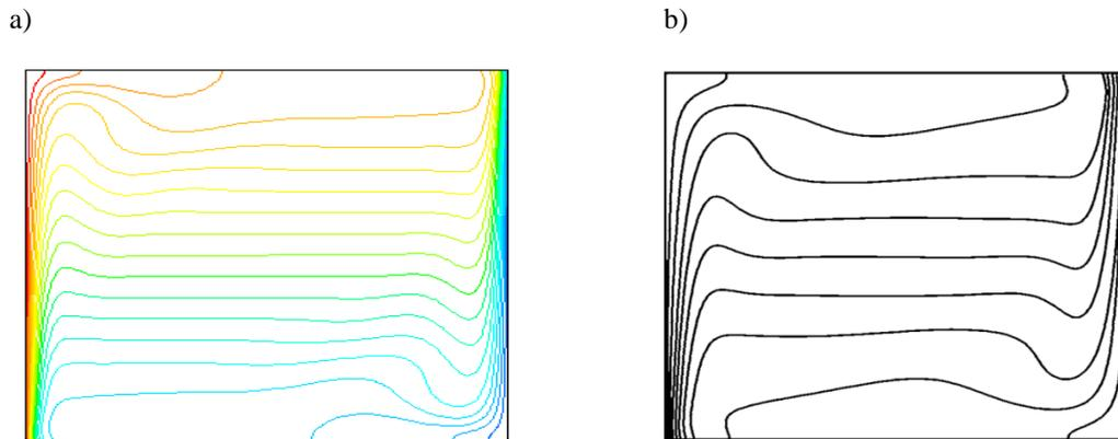
**Figure 12:** Thermal field: a): This study, b): experimental results of Wang H and al[9].
