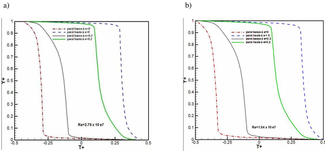
Figure 6: Temperature profiles for different emissivity. a): near the floor; b): near the ceiling
