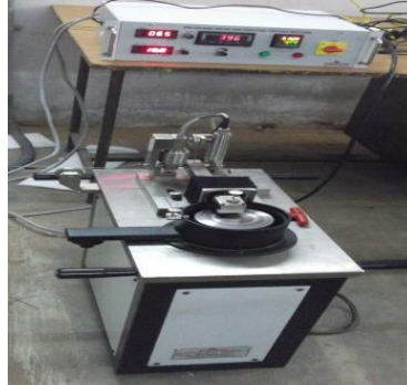
Figure 2: Pin on disc friction monitor
