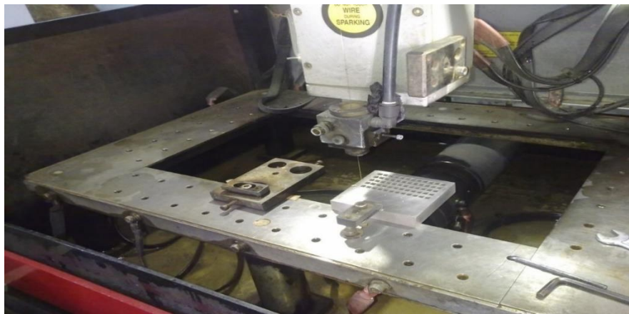
Figure 2:Monel K- 500 Plate Mounted on WEDM Machine
