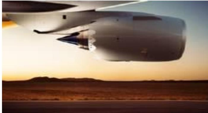
Figure 4: Saw tooth pattern improves noise profile of the Lufthansa 747-8
