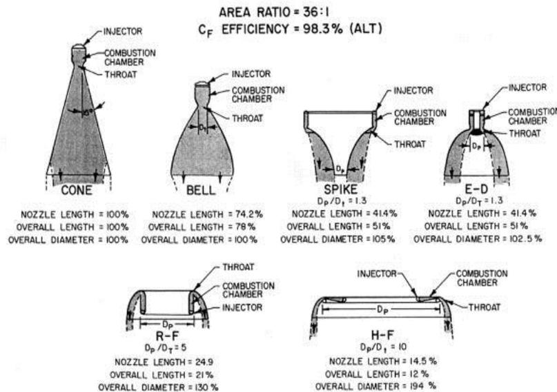
Figure 3: Different shapes of nozzle
