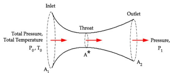
**Figure 2:** Flow through C-D nozzle
