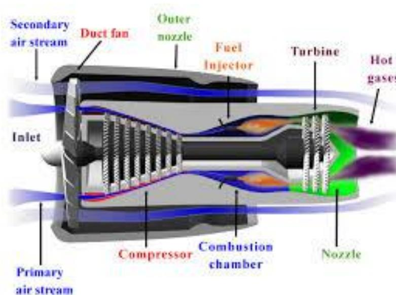
**Figure 7:** Schematic of turbofan engine
