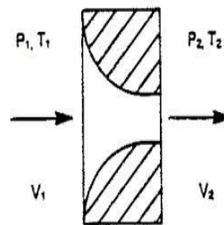
**Figure 1:** Flow through convergent nozzle
