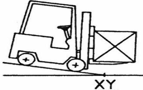
Fig.2. Forward tip over stability while travelling
