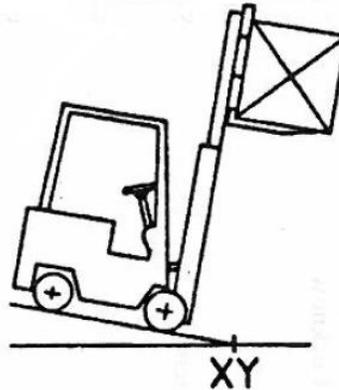
Fig1. Forward tip over stability while stacking
