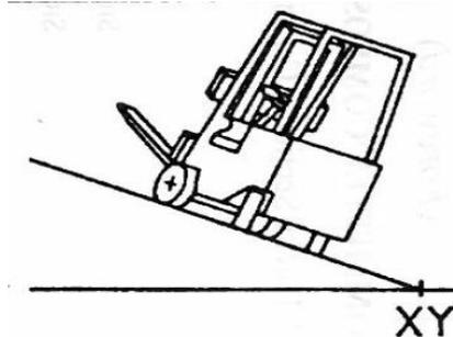
Fig.4. Side tip over stability when empty
