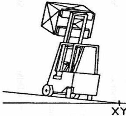
Fig.3 Side tip over stability when loaded
