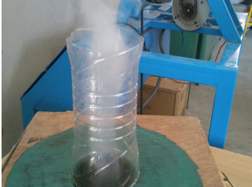
Fig. 4 Visualization of vortex by smoke
