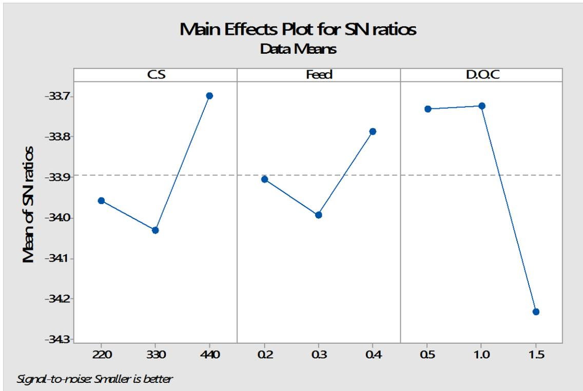
Fig shows the effect of different parameters on Signal o noise ratio
