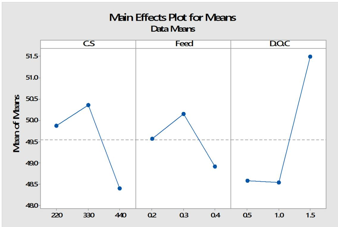
Fig shows the effect of different parameters on MRR
