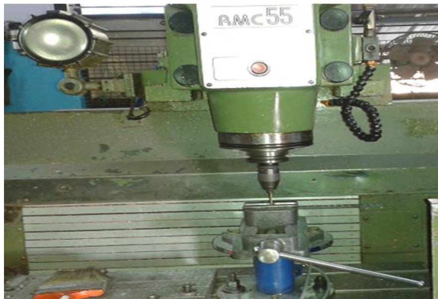
Figure 3: Drilling of hybrid composite fixed on the IEICOS drill tool multi-component piezoelectric dynamometer
