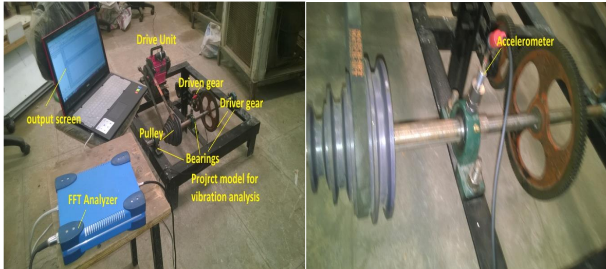
Figure.3: Model testing for vibration by using NV-Gate FFT analyzer
