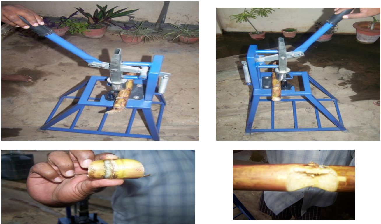
Fig: 6.2. Working prototype of the sugar cane bud chipping machine
