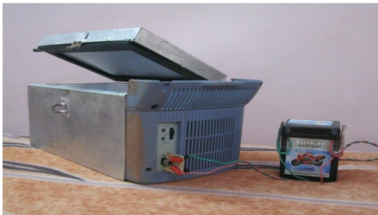
Fig 6.6: Fabricated model of the Thermoelectric Vaccine Preservator with battery attached.
