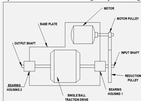
Fig.4 Test Rig for the Analysis of Performance characteristics
