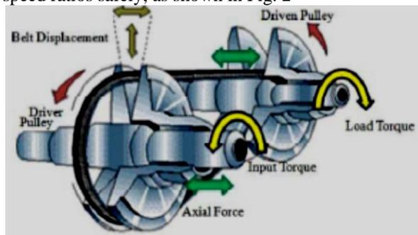
Fig. 2 Model of metal V-belt CVT.
