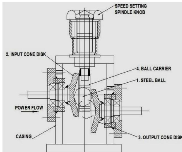
Fig.3 Principle of Operation of Single Ball Traction Drive
