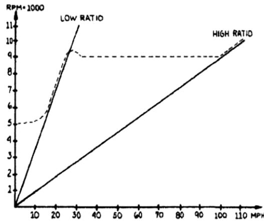
Fig.1 CVT Curve for Engine Speed and Velocity of the Vehicle
