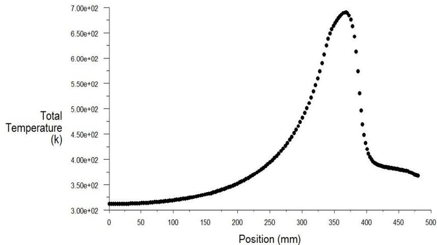
**Figure 9: Temperature distribution of Stainless steel top wall**
