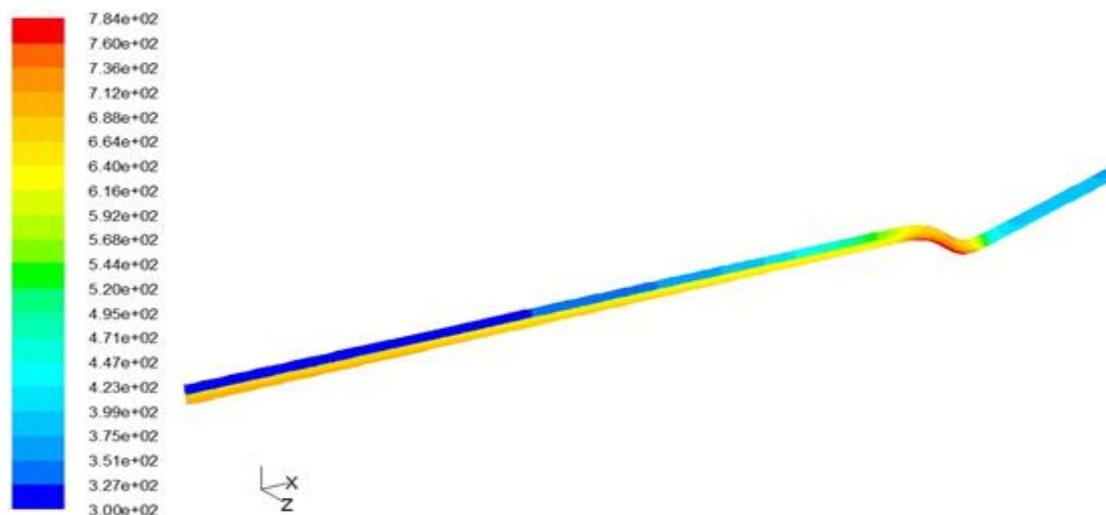
**Figure 4: Three-dimensional schematic of computational domain and converged contour for total temperature**
